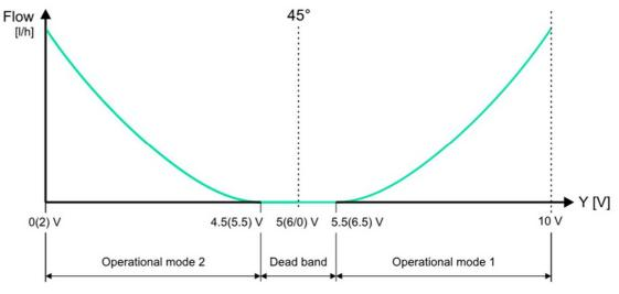
Note: Values in brackets refer to a 2...10 V control signal, e.g. 0(2). (6/0) - with a 2...10 V control signal, the actuator drives the valve to the closed position (45°) for open Y signal input (0 V).
