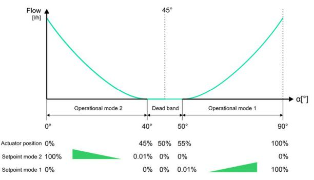
Cooling and heating allocation is freely selectable. However, Siemens suggests an equal allocation for all valves during installation for safety reason as below:
