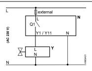
controller (thermostat) actuator with zone valve system potential AC 230 V Y L Ν system neutral control signal OPEN
