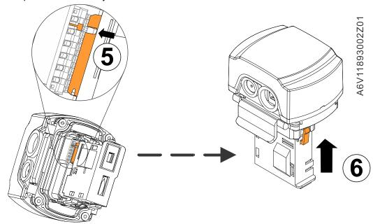
4. Install the sub-housing on the main housing.
