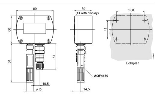
Dimensioning without (with) LCD-display Dimensions in mm
