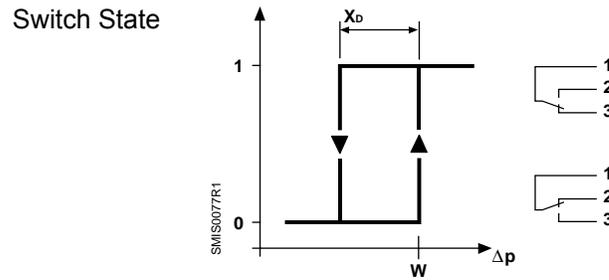
Figure 1. Operation Diagram.
