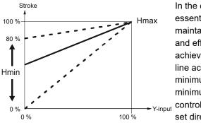
In the case of a suction throttle valve, it is essential that a minimum stroke limit be maintained to ensure compressor cooling and efficient oil return. This can be achieved with a reinjection valve, a bypass line across the valve, or a guaranteed minimum opening of the valve. The minimum stroke can be defined via the controller and control signal Y, or it can be set directly with potentiometer Rv.
