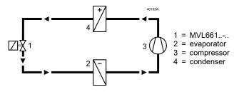
Electronic superheat control is achieved by using additional control equipment (e.g. PolyCool).
