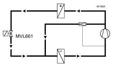
Note A larger valve may be required for low load operation than is needed for full load conditions. To ensure that the selected valve will not be too small for low loads, sizing should take account of both possibilities.
