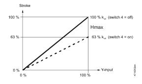
For  $k_{vs}$  reduction (DIL switch 4 in position ON), the stroke is limited to 63% mechanical stroke. 63% of full stroke then corresponds to an input/output signal of 10 V. If, in addition, the stroke is limited to 80%, for example, the minimum stroke is 0.63 x 0.8 = 0.50 of full stroke.
