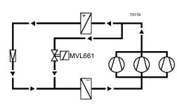
Suitable for use in large refrigeration systems in air conditioning plant, to prevent unacceptable temperature fluctuations between the compressor stages.
