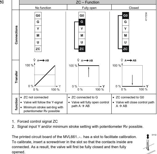
Calibration matches the electronics to the valve mechanism. During calibration, the green LED flashes for about 10 seconds; refer to "Indication of operating state" (page 5). **MVL661..-.. refrigerant valves are supplied fully calibrated.**
