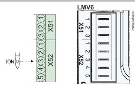
Measuring circuit for detector current measurement
